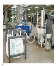
We manufacture a Pressure conveyor appropriate for feeding powder filling system with empty capsules and machines with full capsules, without opening or changing its integrity. These products are coated with stainless steel and have almost no noise level. Size is portable and could be used in small of area. The volume of container is 200 Lit.
